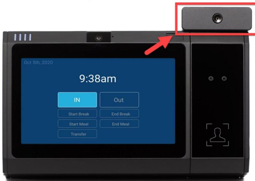
This thermal scan uses a default temperature threshold of 102° F. If the employee's temperature is above that threshold (not equal to), the punch process is interrupted, they are instructed to contact their manager, and their punch is not recorded. The thermal scan occurs every time an employee uses the clock, including when they clock out.
