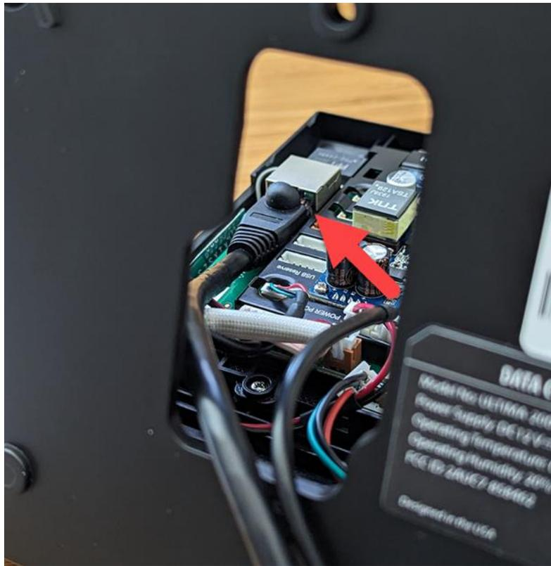
3. **Power up the clock.** With the clock still open, run the DC power connector from the clock's circuit board through the opening on the back of the clock. Connect it to the power supply and plug in the clock. The clock will boot to the registration screen automatically. There is no ON/OFF switch for the clock.
